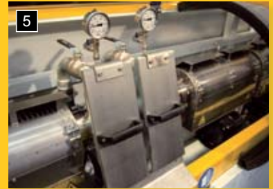
Simple degassing with two maintenance covers
