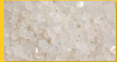
Pellets produced from PE film
