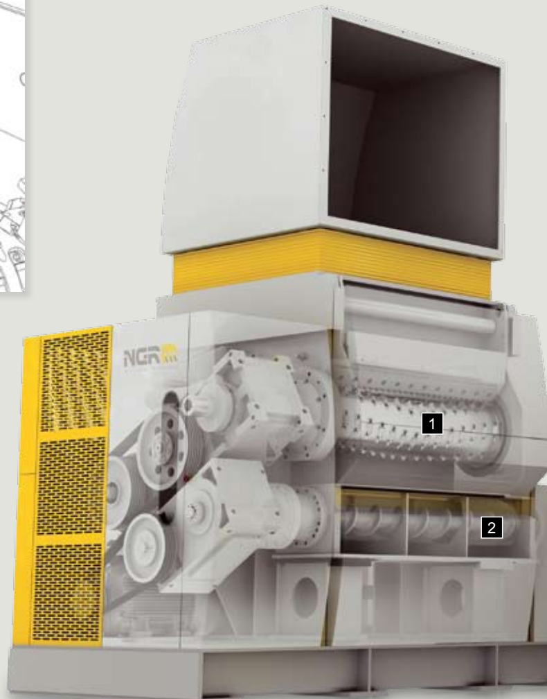
The hydraulic ram pusher presses the material against the shredder.
