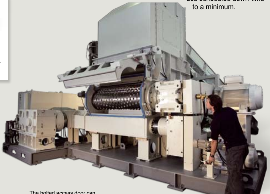
The bolted access door can be opened and closed hydraulically.
